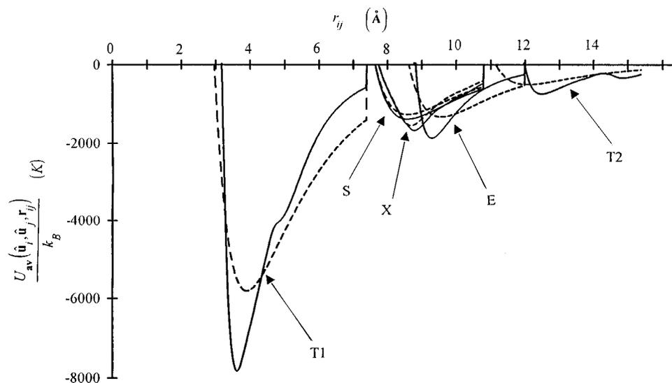
FIG. 1.  $U_{av}(\hat{\mathbf{u}}_i, \hat{\mathbf{u}}_j, r_{ij})$  data (solid lines) for the azimuthally averaged interaction potential of *p*-terphenyl and triphenylene, and associated fit of the generalized Gay-Berne model (dashed lines). See text for fit parameters. The fits were generated using data from a limited range of  $r_{ij}$  values; the upper limit of this range, for each of the curves shown, is indicated by the vertical discontinuity at large  $r_{ij}$ .
